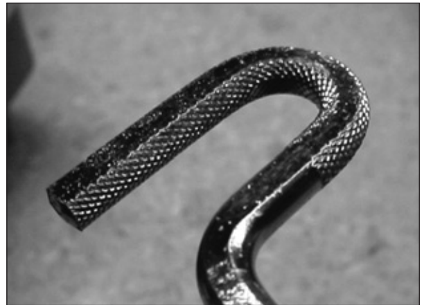
2. This knurled tip eliminates tool slippage.
